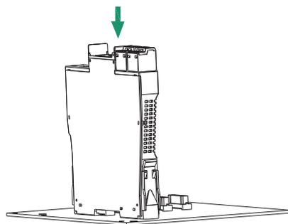
Install the apparatus, make the both sides of the apparatus aim at the slot of the backplans, press down the apparatus onto the backplans as the direction of the arrow.
